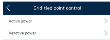
Figure 7-11 Grid-tied point control
