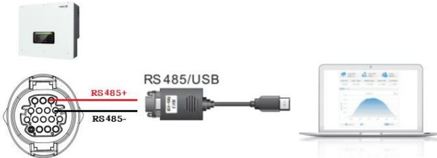
If you need to use upper computer software, please consult the after-sale technical support personnel of SOFAR SOLAR. The upper computer software can be used to set the enabling and parameter of power control, over and under voltage load shedding parameters , over and under frequency shedding parameters, and reactive power output enabling and parameter setting.
