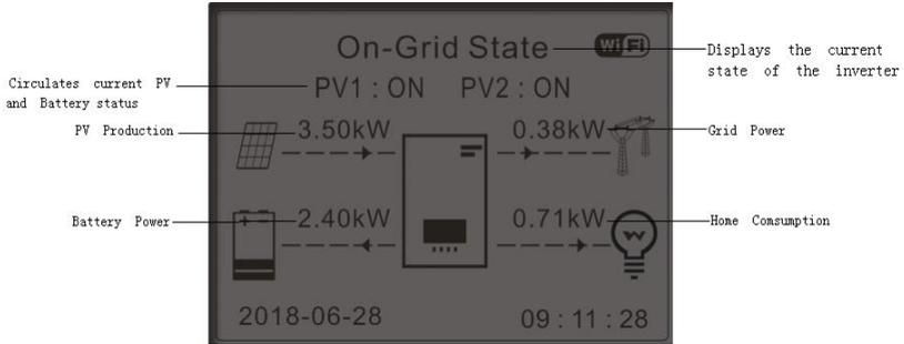
In the main interface, press “Down” button to enter grid/battery parameters page.
