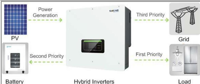
**Power Consumption Priority Level: Load > battery > grid**
