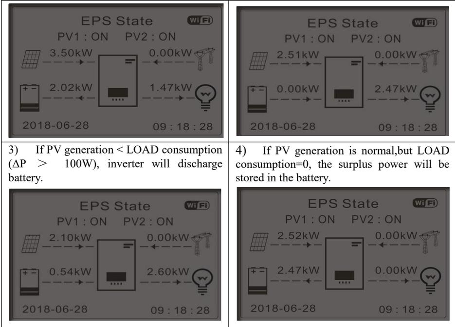
3) If PV generation < LOAD consumption ( $\Delta P > 100W$ ), inverter will discharge battery.
