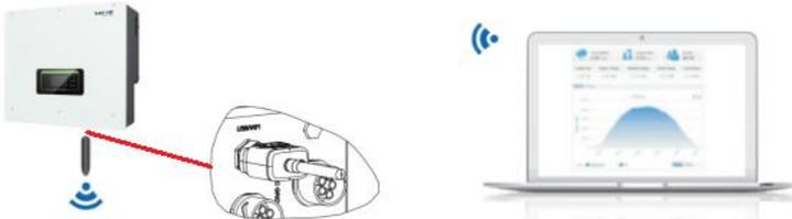
The operation information (generated energy, alert, operation status) of the inverter can be transferred to PC or uploaded to the server via WiFi/GPRS. Users can choose to use web or APP for monitoring and viewing according to their needs. They need to register an account and bind the device with the WiFi/GPRS SN number. The SN number of the WiFi/GPRS shall be affixed to the package box and the WiFi/GPRS.
