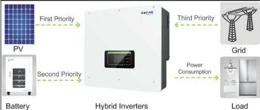
**Power Supply Priority Level: PV power > battery > grid**
