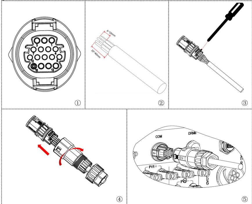
Please refer to the following figure for RS485 connection When you need to use RS485 as a cascade of monitoring between inverters.
