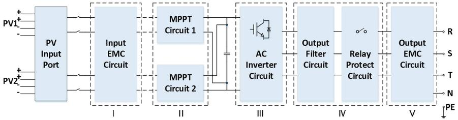
Figure 2-8 Schematic diagram
