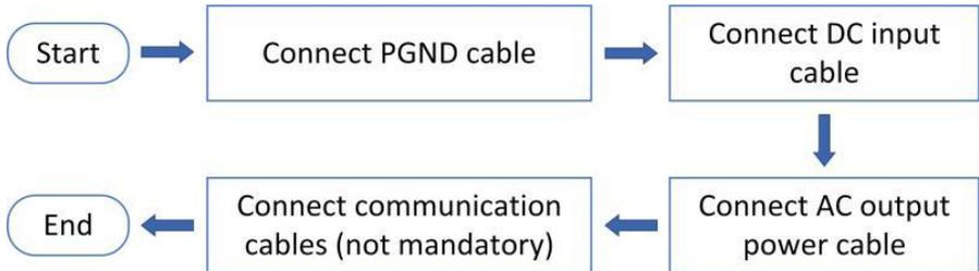
Figure 4-1 flowchart for connecting cables to the inverter
