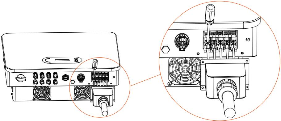
Figure 4-10 AC cable connection instruction diagram (2)
