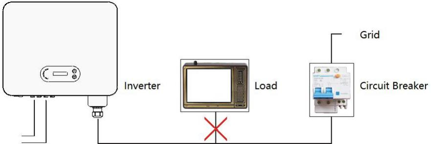
Figure 4-5 Incorrect connection between load and inverter
