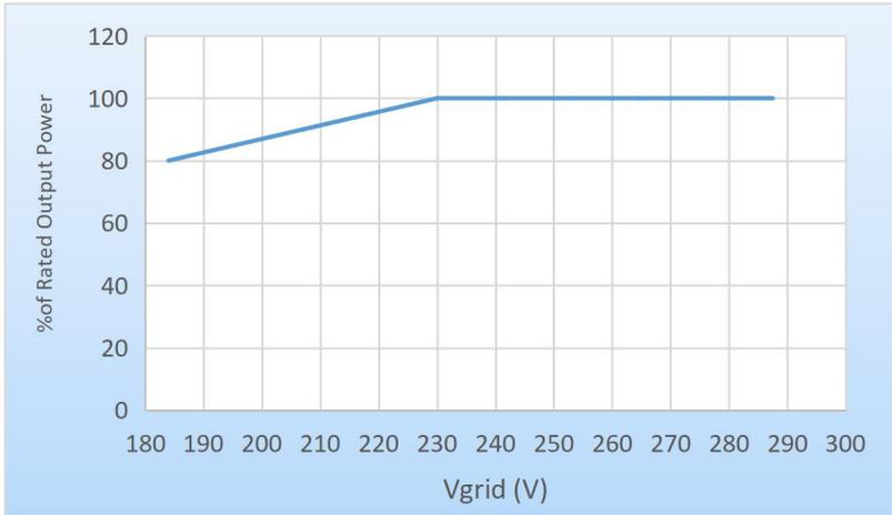
Figure 2-10 Rated Power ratio vs Grid Voltage
