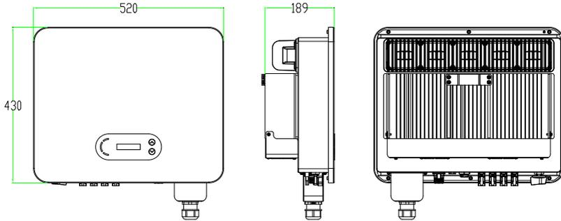
Figure 2-3 Front, side and back of the machine (15~24K)
