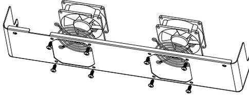
Figure 7-2 remove the fan and protective cover
