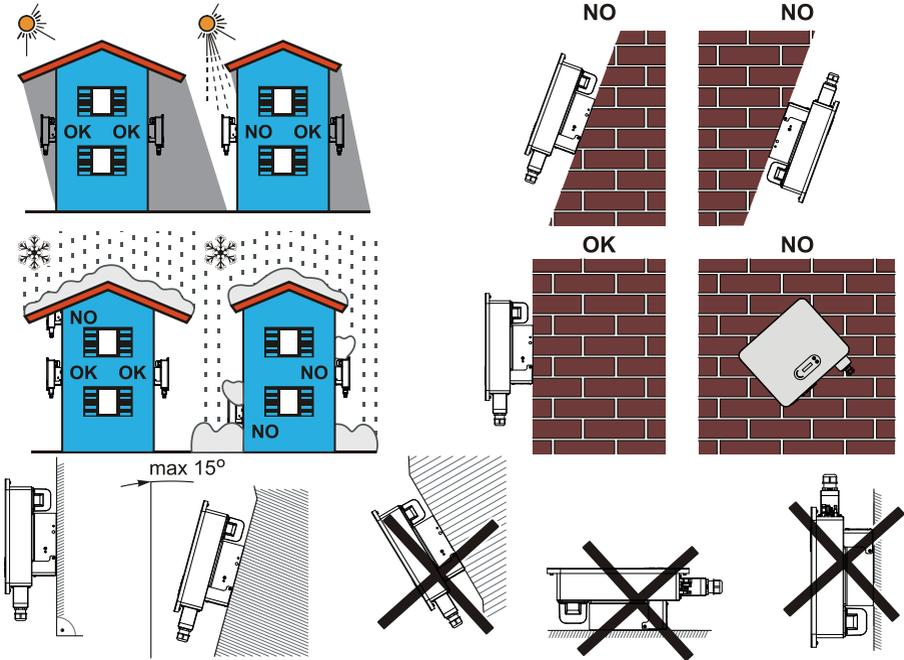
Figure 3-1-Installation Position Selection
