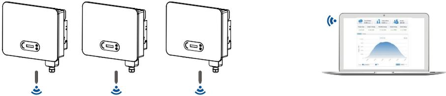
Figure 4-22 Connect multiple USB acquisition stick (WiFi version) to wireless router
