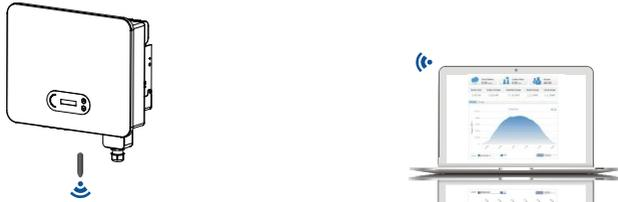
Figure 4-21 Connect one USB acquisition stick (WiFi version) to wireless router
